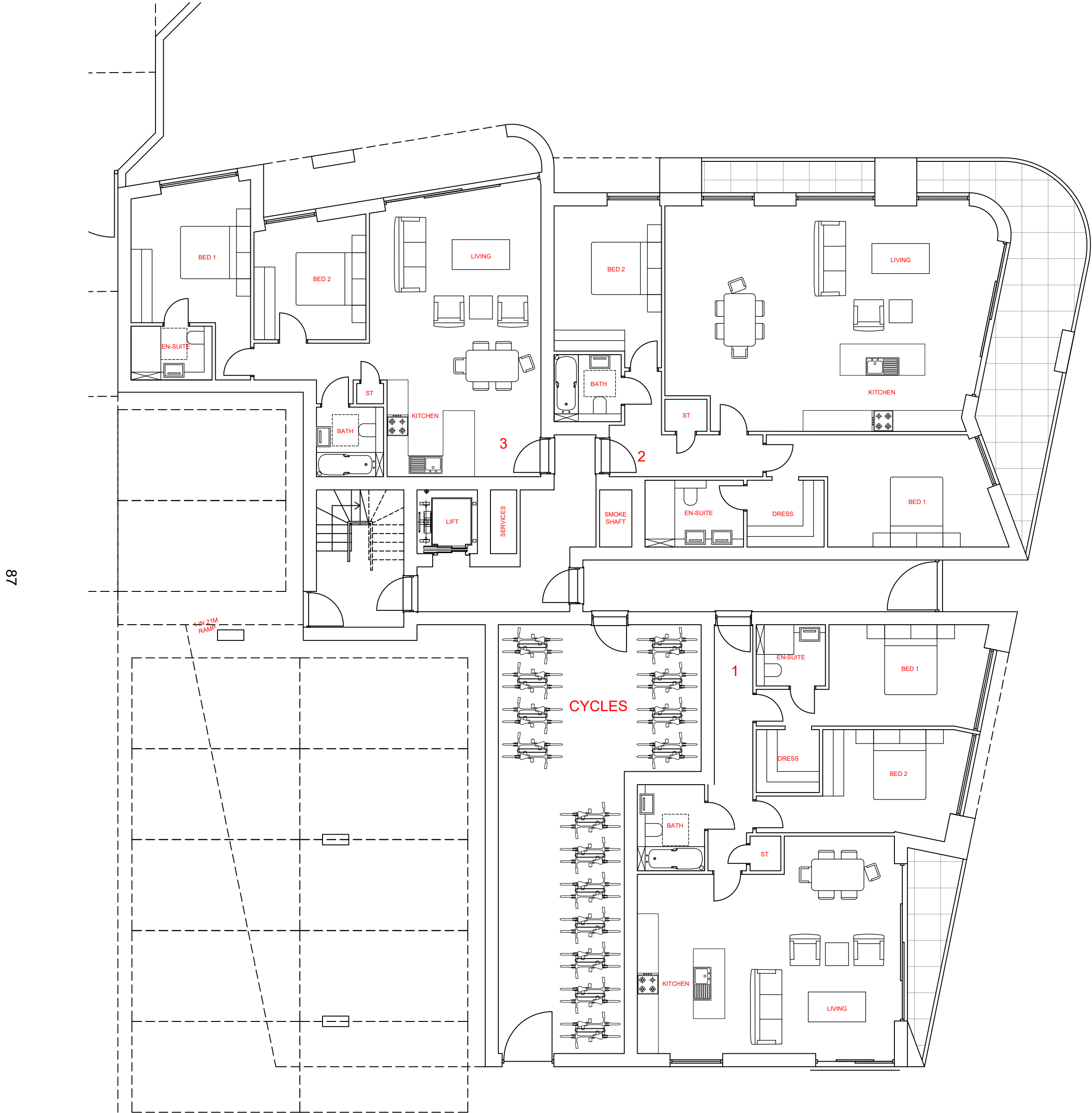
GROUND FLOOR PLAN: SCALE 1:100
